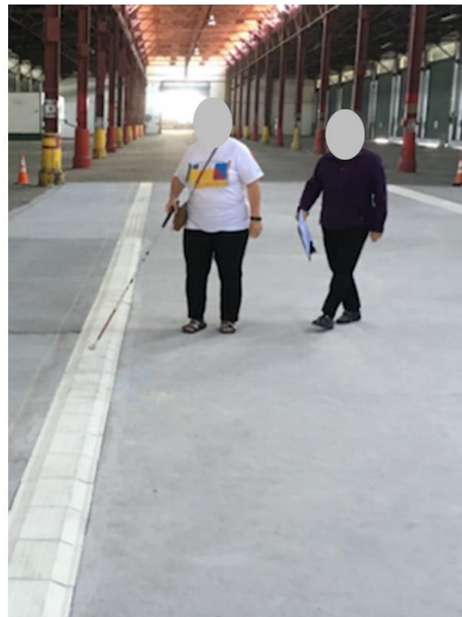
Figure 6. The left panel is drawings of the trapezoidal TWD in top view and cross section. The right panel is a photo of a research participant who was blind detecting the TWD with their long cane. An orientation and mobility specialist is nearby to ensure participant safety. [Sources: Drawing, L. Tabor; photo, B. Bentzen]
