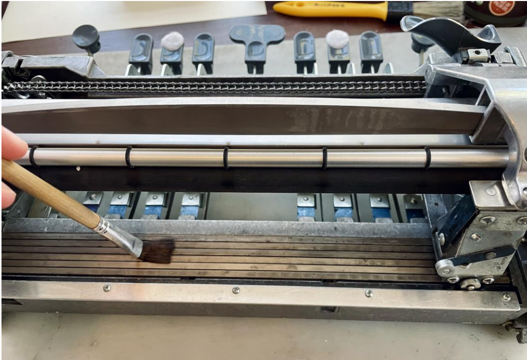
Figure 4.1.2 Top interior view. Oil is applied to the length of the cam rods.
