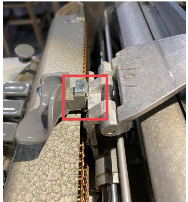
Figure 5.4.2 Correct placement of plastic knob.
