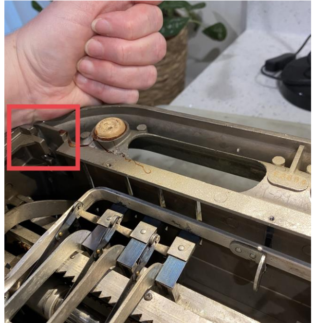
Figure 5.3.1.2 Bottom interior view of front after smashing apron into place
