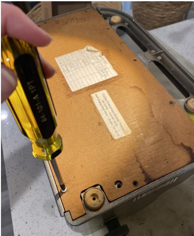
Figure 5.8 View of Bottom cover being reattached to Perkins brailleur
