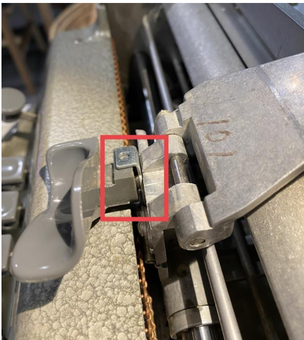
Figure 5.4.1 Incorrect placement of plastic knob.
