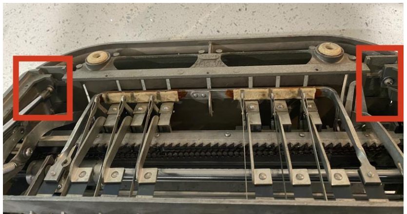
Figure 1.7.2 interior bottom view showing apron screw locations
