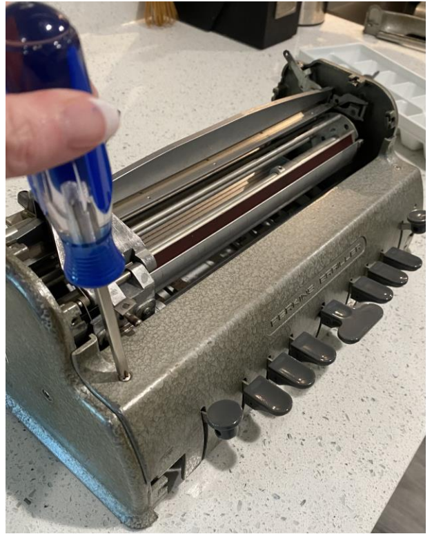
Figure 1.8 Top view, removing front cover
