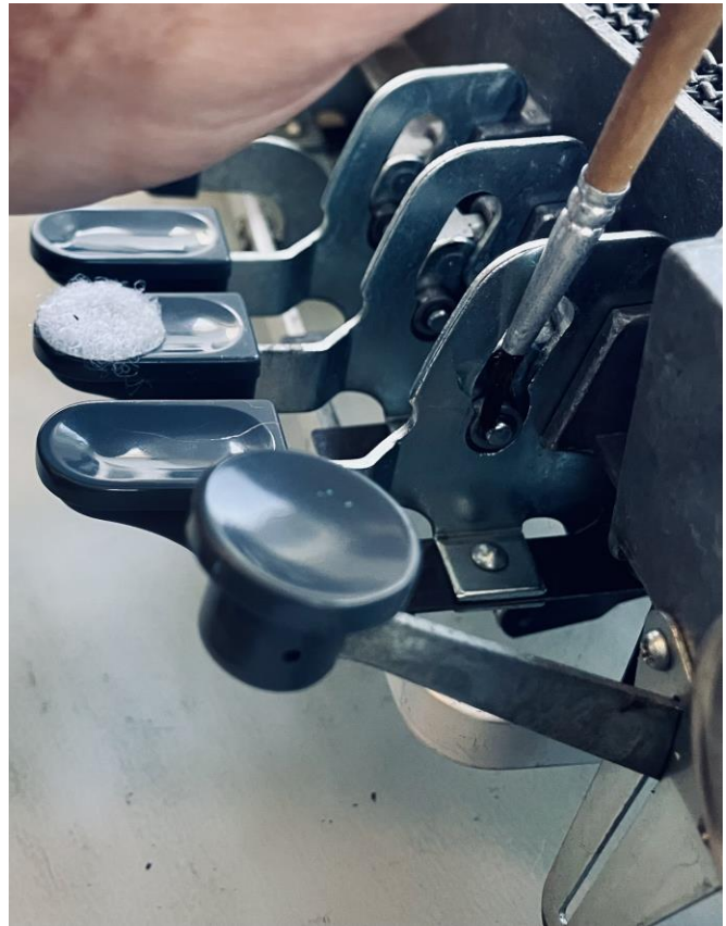
Figure 4.1.3 Front-right interior view . Oil is applied to the top of each cam roller.
