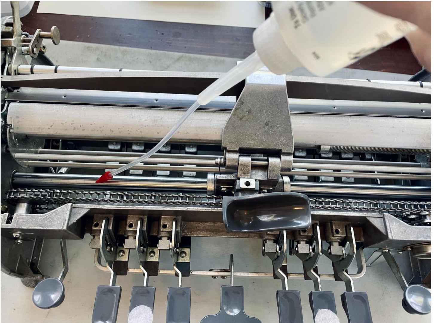
Figure 4.1.1 Demonstration of sewing machine oil application to carriage tube.
