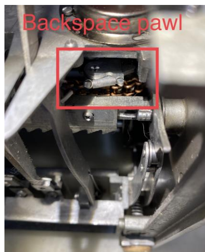
Interior bottom view, right side-backspace pawl
