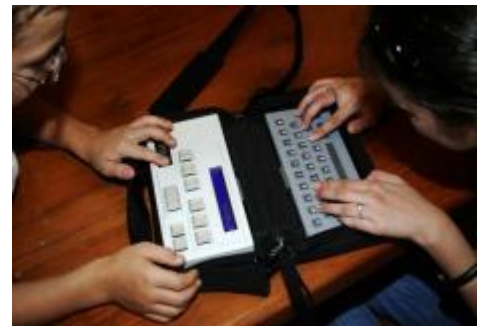
Figure 23 Two people use technology to communicate with each other using braille and print.
